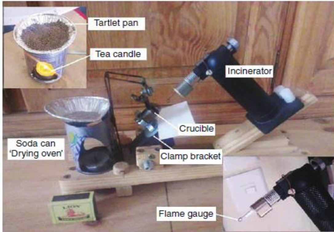
Estimating soil carbon. Rapid Incineration Field Test (RIFT), Albert Ackhurst, Raymond Auerbach, Josua Louw, Nelson Mandela University, George, South Africa. From chapter 17 in the book « Organic Food Systems – Meeting the Needs of Southern Africa»
